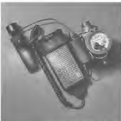
Figure 16.1 Water meter with remote monitoring computer
